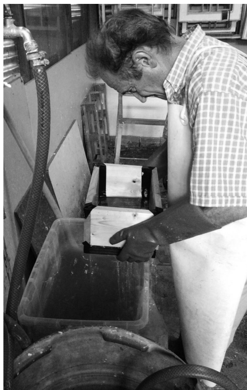
..... Juan lifts the deckle and screen while the water drains. (Bill Horne photo)
