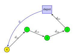
Figure 3: Resulting Cycle from the Vehicle Routing Problem Example
