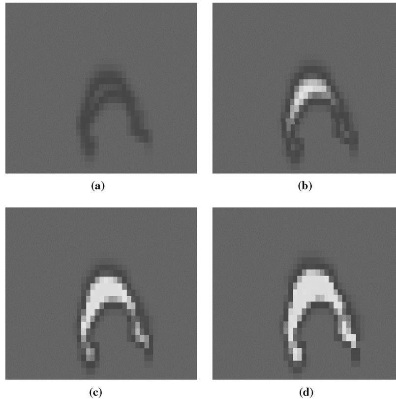
Fig. 16. Over-abstraction and reduced aquifer levels provoke sea water intrusion and aquifer salinisation after (a) 15 months, (b) 30 months, (c) 45 months, and (d) 60 months.
