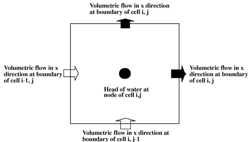
Fig. 9. A schematic representation of the flows calculated for each cell in the aquifer.
