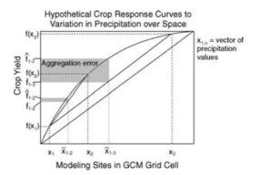
Fig. 1. Hypothetical aggregation error by up-scaling non-linear relations between crop yield and precipitation (Source: Easterling [19]).
