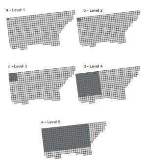
Fig. 4. Cluster (square) aggregation method.
