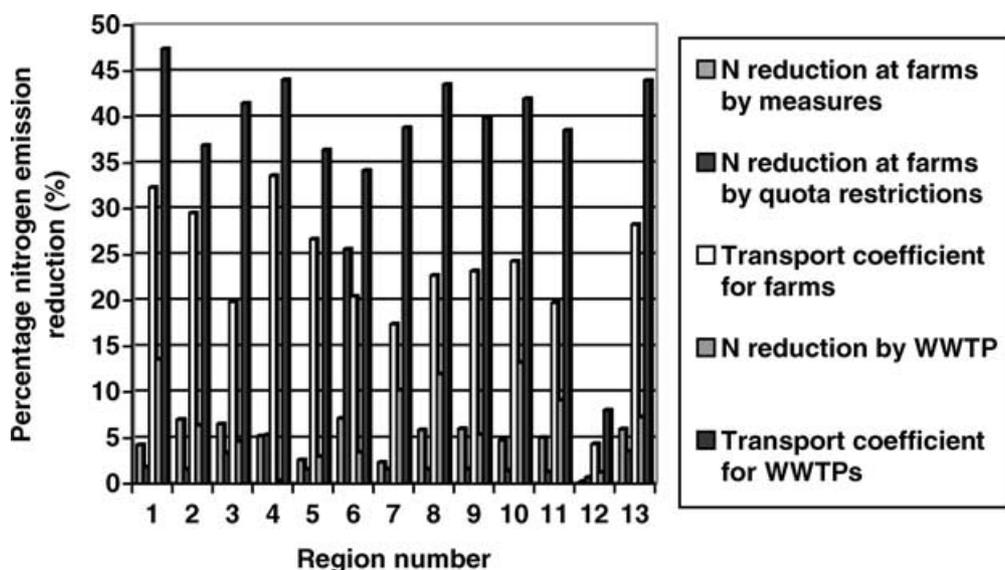
Fig. 4. Percentage N emission reduction in the various regions in a cost-effective allocation. Target is a 30% reduction in nutrient loads to the North Sea (for region numbers, see Table 3). Also the transport coefficients are represented (for agricultural sources multiplied by 100, for WWTPs by 50).
