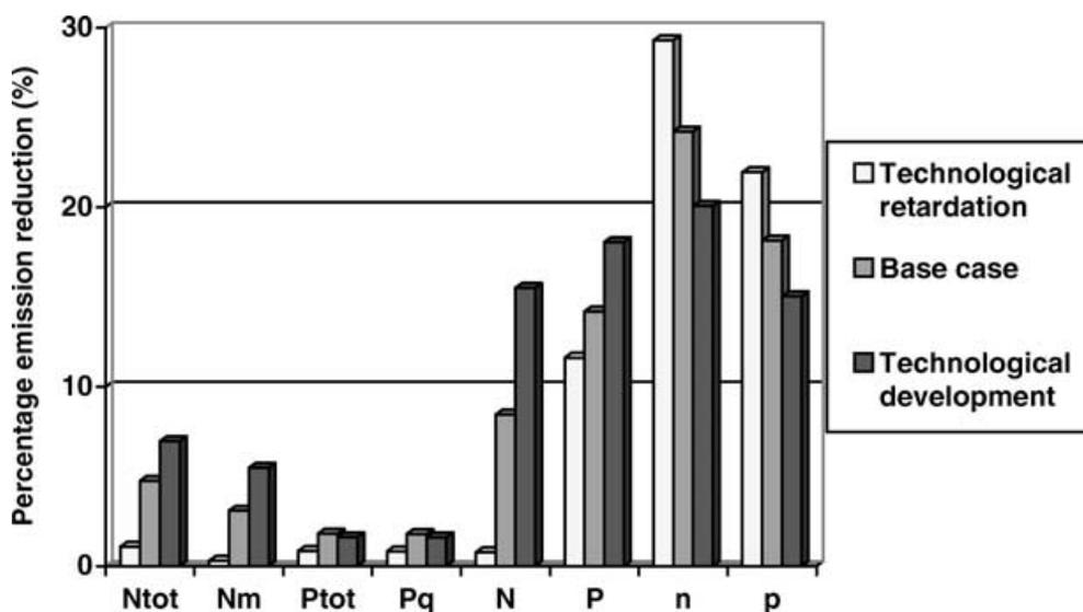
Fig. 8. The impacts of changes in technological development on nutrient abatement measures in the Rhine basin in a cost-effective allocation of 30% reduction in loads to the North Sea.
