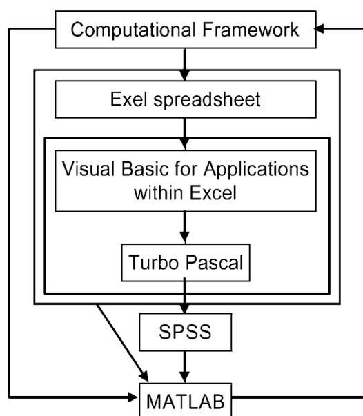
Fig. 2. The interaction between software packages.
