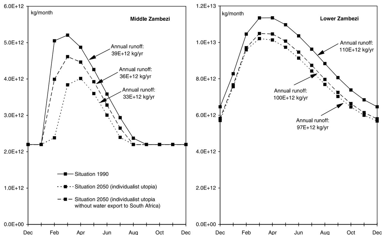
Fig. 8. Changes in the hydrographs for the Middle and Lower Zambezi basins in the individualist utopia. The effect of water export to South Africa is shown by presenting hydrographs for both the case with export and the case without export.
