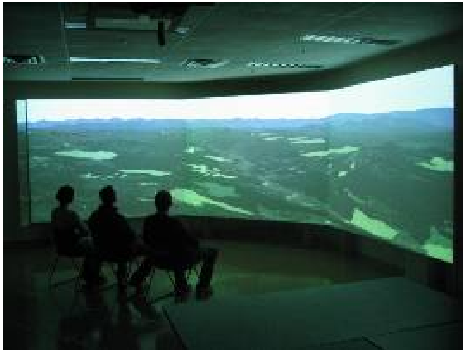
Figure 6: An immersive visualisation environment which can present life-size panoramic imagery on large wrap-around screens, sometimes to dramatic effect. CREDIT: CALP, UBC.
